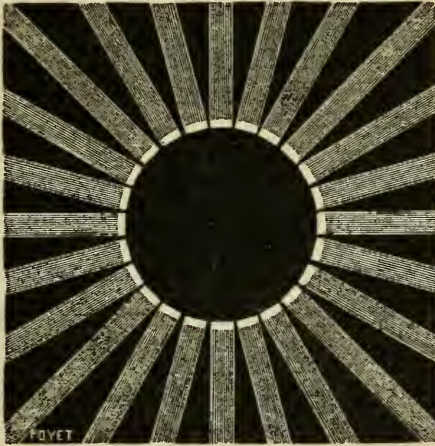
FIG. 4.—A TWENTY-FOUR PANEL LIGHT, WHICH WAS INTRODUCED INTO CERTAIN FRENCH LIGHTHOUSES.
